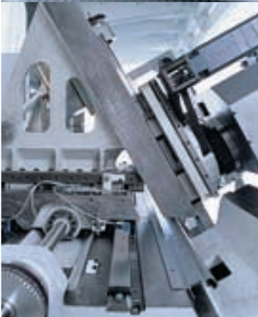
B-axis, Y-axis realized above a wedge slide.
