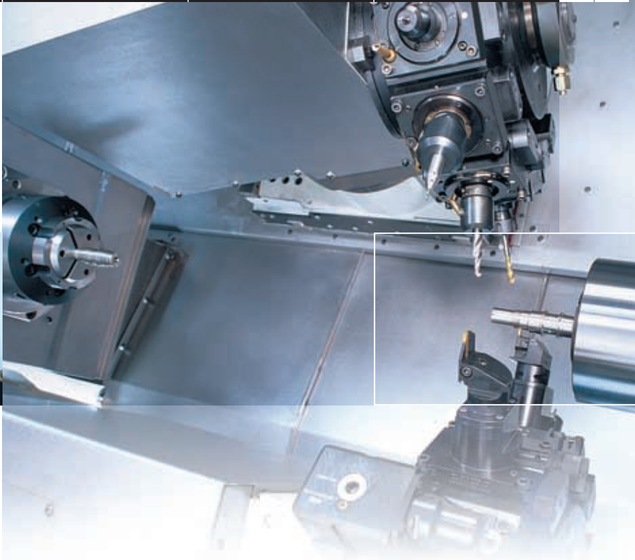
Machining with driven tools.
