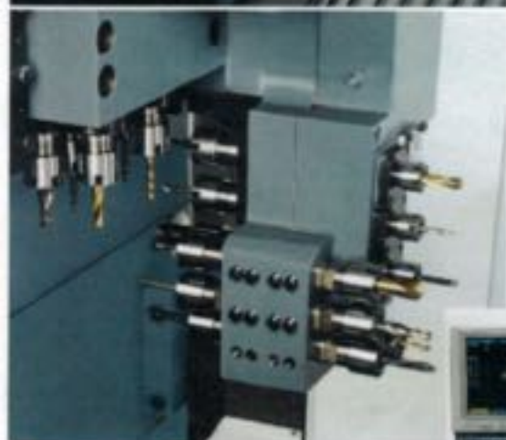
Using Live Bushing with Guide Bushing
